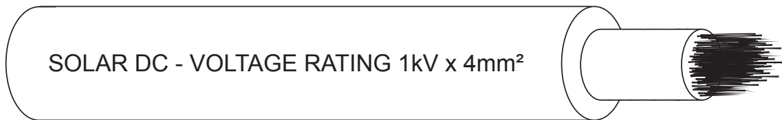
Figure 8: Double insulated solar dc cable
